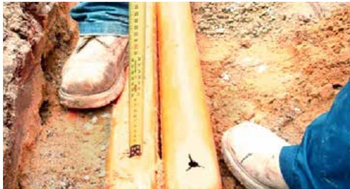
*Pipe damaged by a star dropper*
