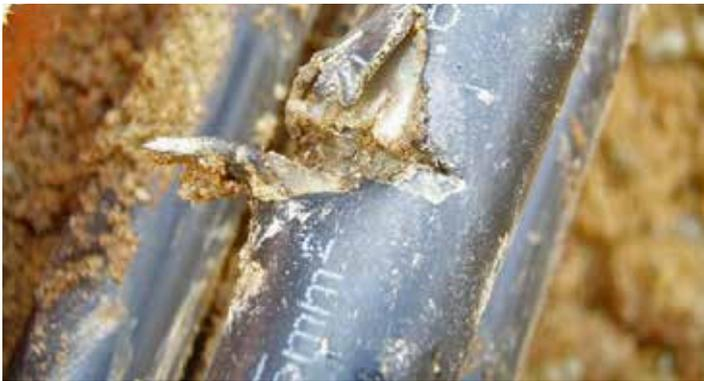
*Cable damaged by an excavator*
