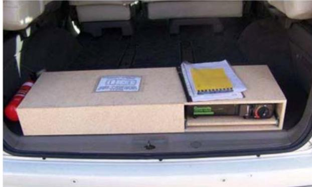
An unsecured camping stove and storage compartment, as shown above, do not constitute an acceptable conversion.
