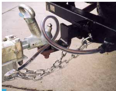
An over-ride braking system as part of trailer coupling
