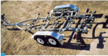
Three types of trailer - the multi-roller type (above), a combination of rollers and skids (below) or one fitted only with skids
