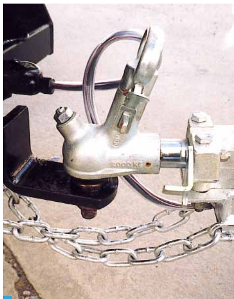
Safety chains in place and correctly fitted
