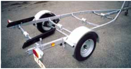
Three types of trailer - the multi-roller type (above), a combination of rollers and skids (below) or one fitted only with skids
