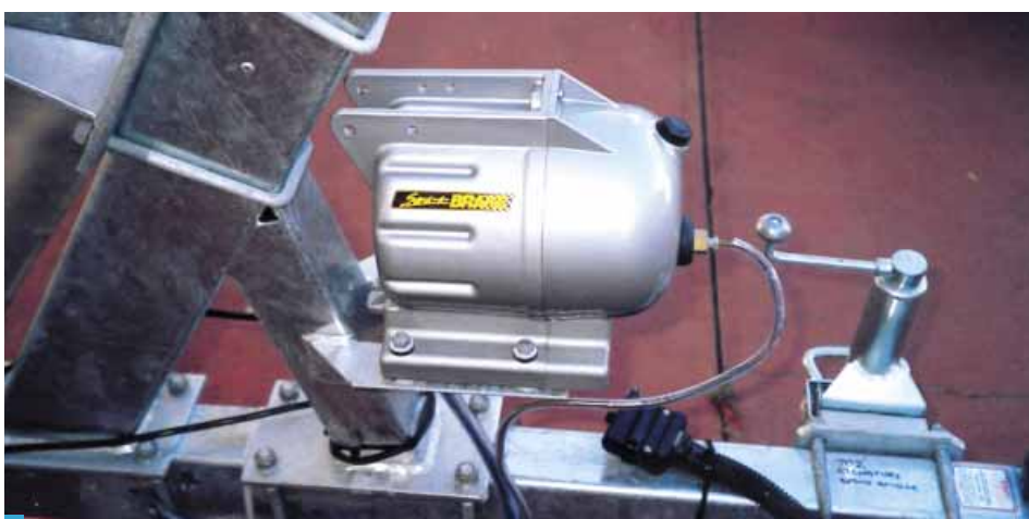
Examples of braking systems. Above, a vacuum-assisted hydraulic system. Below, a ratchet handbrake system (left) and the cable connection to the wheel (right)
