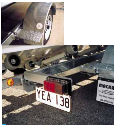
A trailer with correctly-fitted submersible lights and one side reflector
