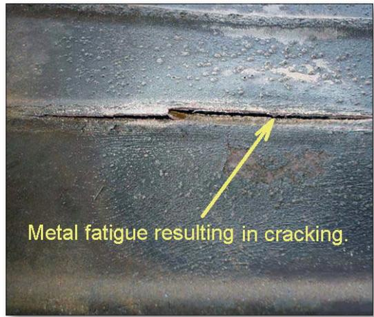
Metal fatigue and cracked heat exchanger
