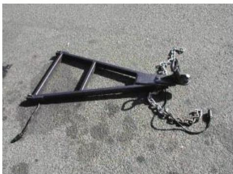
Figure 1: Typical A-frame with safety chains fitted
