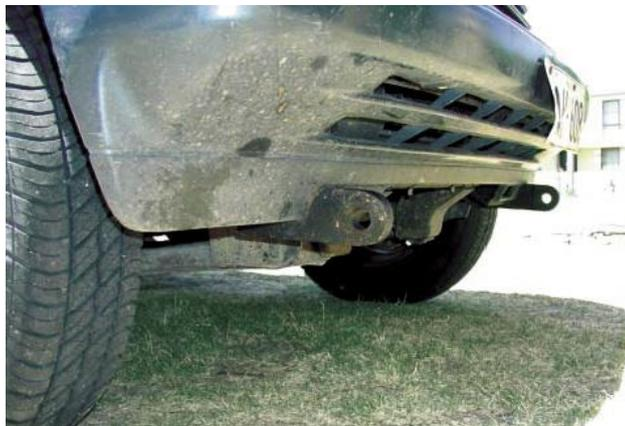
Figure 2: Attachment points for A-frame
