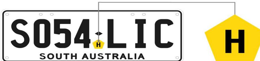
Figure 2: example label for hydrogen-powered vehicles
