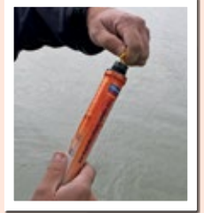
Step 2: Hold flare by handle at bottom, pull tab up and out quickly and firmly.
