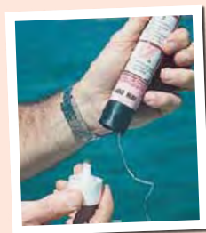
Step 1: Remove the cap from both ends. The bottom cap is the striker. Hold the flare at the base and use the striker to ignite the flare at the top.
