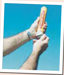
Step 2: Firing lever will drop down. Press the firing lever against the cylinder to fire.
