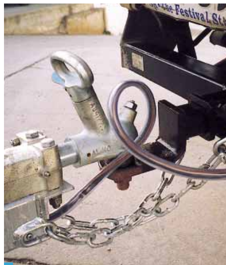
An over-ride braking system as part of trailer coupling
