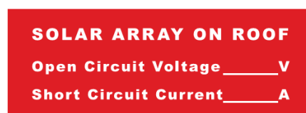
Example of Fire emergency information required at main switchboard (Clause 5.4)
