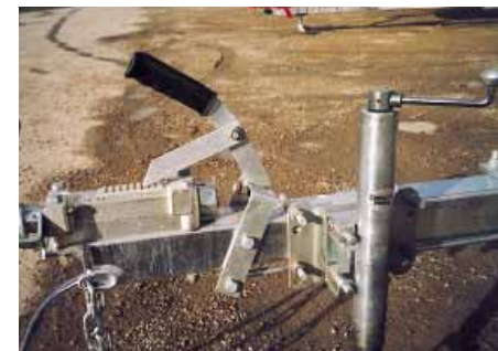
Examples of braking systems. Above, a vacuum-assisted hydraulic system. Below, a ratchet handbrake system (left) and the cable connection to the wheel (right)
