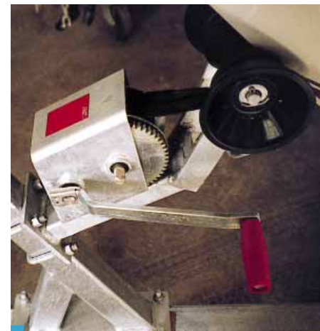
A typical two-speed hand winch
