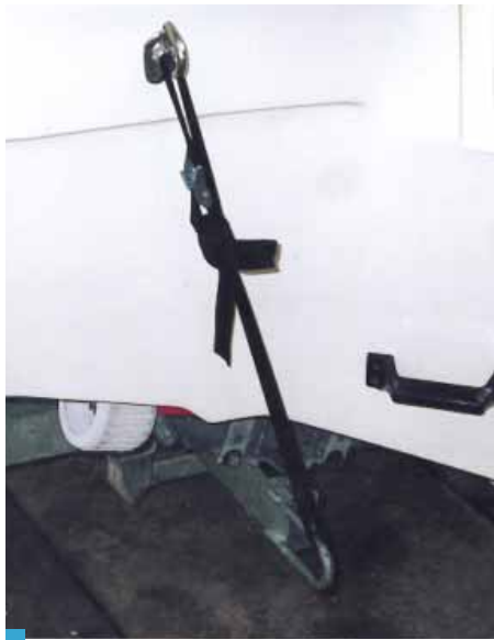
A tie-down holds the boat in place
