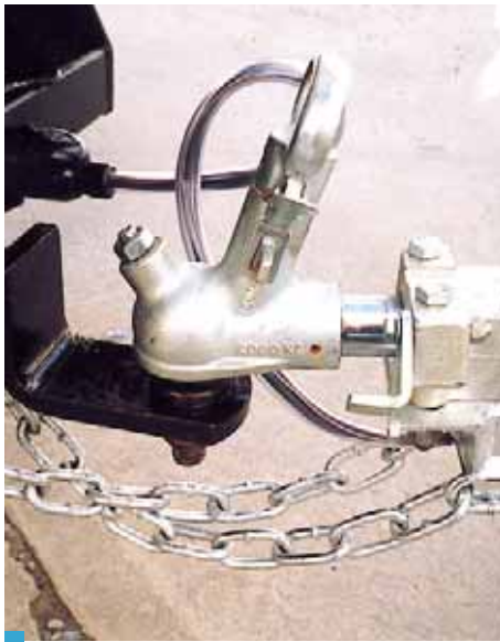
Safety chains in place and correctly fitted
