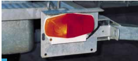
Submersible lights fitted to a boat trailer
