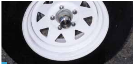
A trailer wheel fitted with a bearing protector
