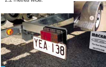
A trailer with correctly-fitted submersible lights and one side reflector
